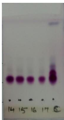
**Fig. 3.** TLC of  $\beta$ -sitosterol derivatized with vanillin sulphuric acid
