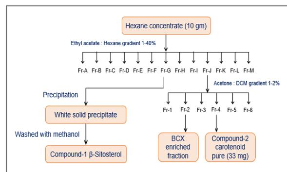
**Fig. 1.** Overall column chromatography
